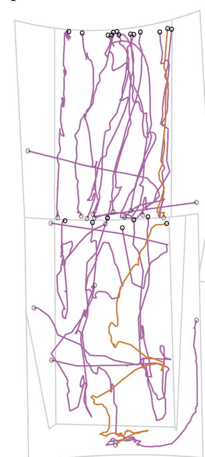
Figure 2: The swimming trajectories of the three species on the barrier were extracted from the video footage of all three tested water discharges by hand. The 130 L/s water discharge is representative for real fish passes. The gray lines represent barrier contours.
